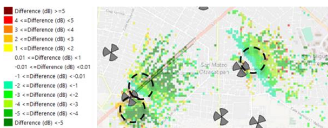
Fig. 5. SINR Improvements with RF re-design and antenna tilt
