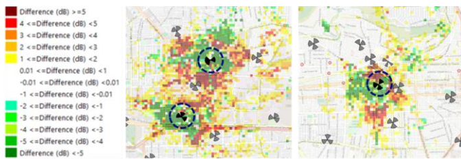
Fig. 4. SINR Improvements with introduction of low band frequency
