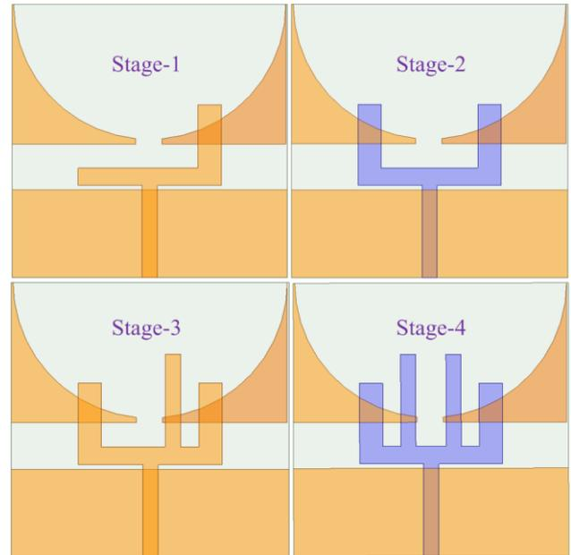
Fig. 3. Different stages of the proposed antenna
