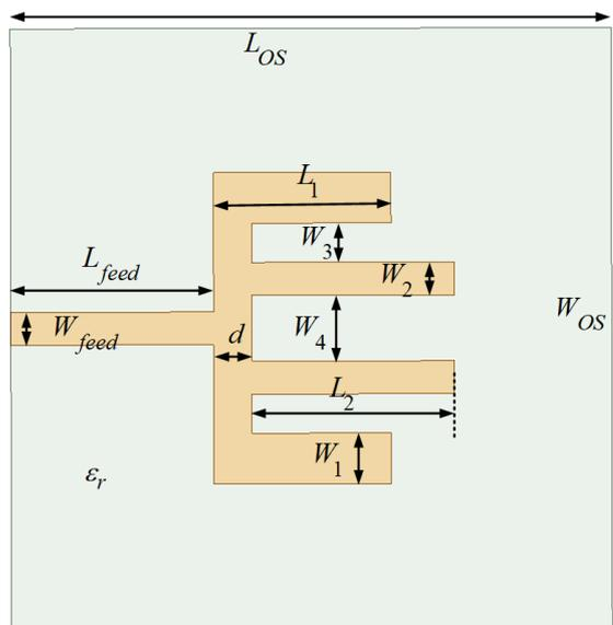
Fig. 1. Top view of proposed UWB antenna
