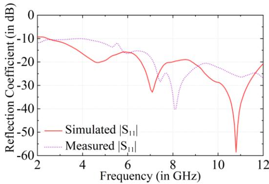
Fig. 8. Simulated and measured reflection coefficient of the proposed antenna
