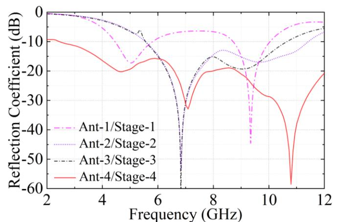
Fig. 4. Simulated results of reflection coefficient of the different stages of the proposed antenna
