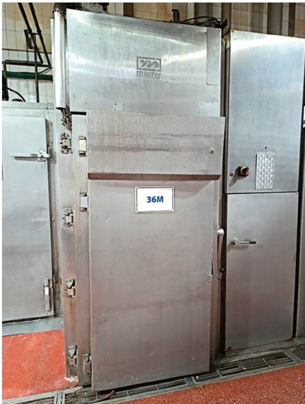
Figure 1. Maurer pasteurisation chamber with one door, which can accommodate two carts
