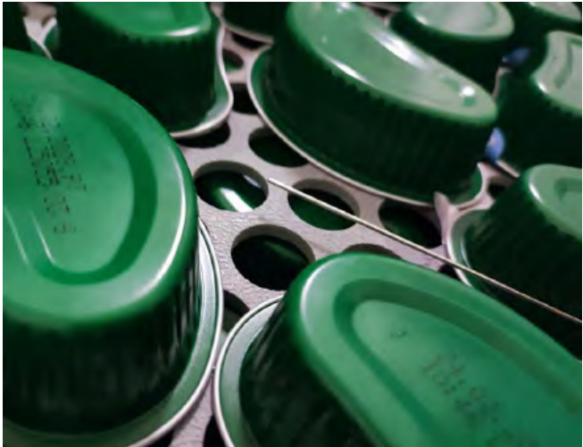
Figure 4. Thermocouple probes placed outside the tuna pâté cans in the carts
