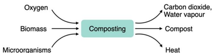
Figure 1 - General representation of composting process Source: Dsouza et al., 2021
