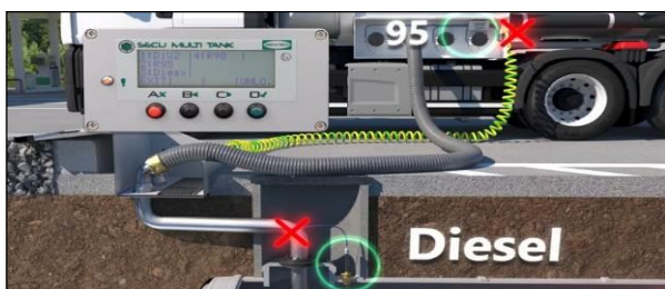
Slika 20 - Prikaz blokade istakanja goriva usled pogrešno povezane instalacije Fig. 20 - Review of blocked unloading due to inadequate connected instalation
