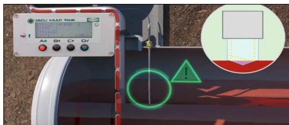
Slika 22 - Prikaz rada senzora pri dostizanju maksimalnog nivoa goriva u rezervoaru Fig. 22 - Review of sensor's work at reaching maximum level of fuel in petrol station tank
