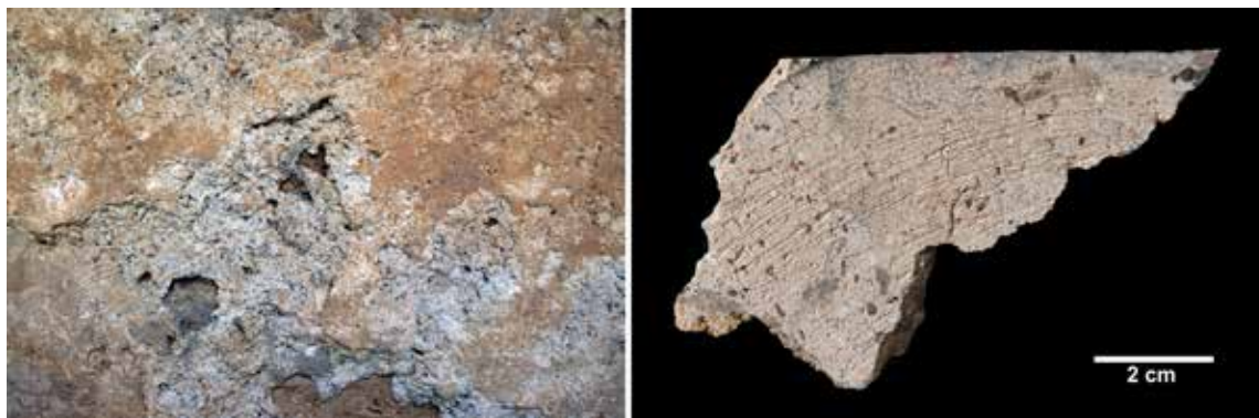
Fig. 4. (left) Ash and charcoal enriched mortar in a Roman cistern from Nora (Sardinia); (right) Cross-section of a sample of an organic ash-rich sample from a cistern render of Nora (photos by Simone Dilaria).
