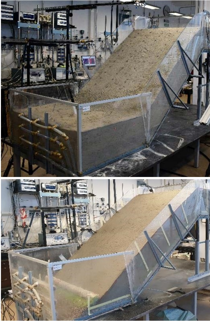
Figure 2 Models with a 35-degree inclination built from clean, uniformly-grained fine sand at the beginning of the test: The case with impermeable bottom boundary condition and the slope's toe reaching the end of the flume (upper photo); The "infinite" slope model over a 5 cm thick layer of gravel to improve drainage conditions - the case considered in this study (lower photo).
