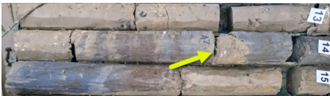
Figure 5. Photograph of BI-3 borehole core log in the zone of the slip surface (yellow arrow)
