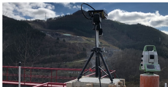
Fig.4. Combination setup radar technology and geodetic technology
