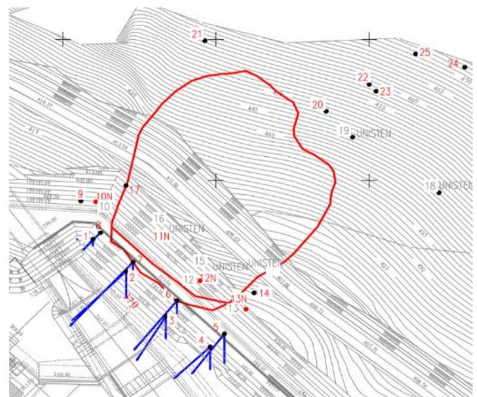
Figure 8 Total horizontal and vertical movements – August 2017
