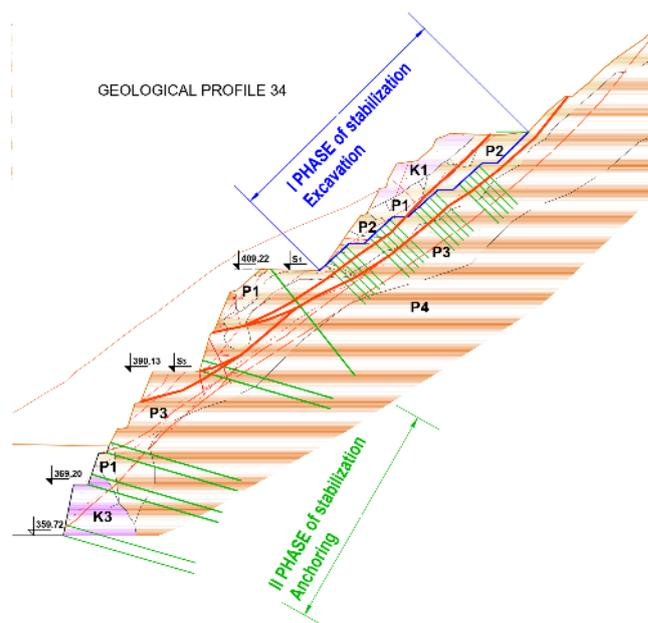
Figure 6 Geological profile 34 with indicated terrain stability measures
