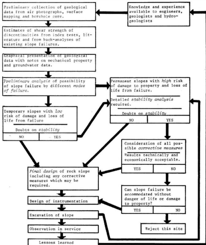
Figure 2 Rock slope design flow chart (Hoek and Londe, 1974)
