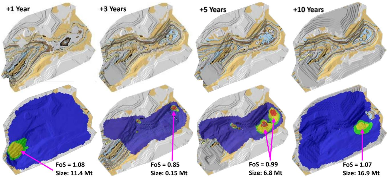
Figure 8 Top: Mine design time horizons with pit progressing from west to east, dumps enlarging and an in-pit dump being constructed. Bottom: Lowest  $FoS$  areas and size of modelled failure mechanisms.
