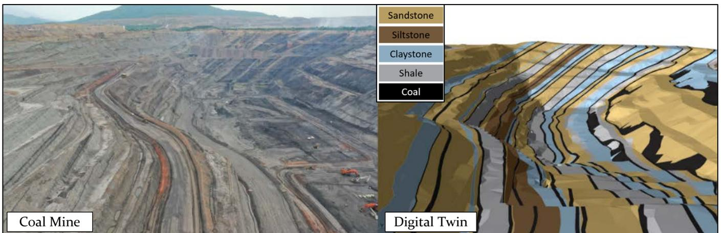
Figure 6 Photograph of coal mine slopes (reality) versus 3D LE model geometry developed in Slide3 software (digital twin) by Rocscience Inc (note: phreatic surface and clay seam interfaces not shown for clarity).
