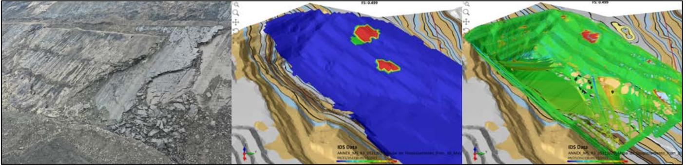
Figure 7 Left to right: Photograph of 30m high failure; 3D LE model outputs (Factor of Safety map: red indicates  $FoS < 1$ ): two multi-bench failures; IDS radar data showing the deformation hotspot associated with the failure in the photograph.
