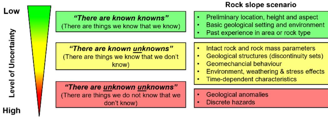
Figure 1 Design uncertainty in association with the geotechnical engineering components for a rock slope scenario
